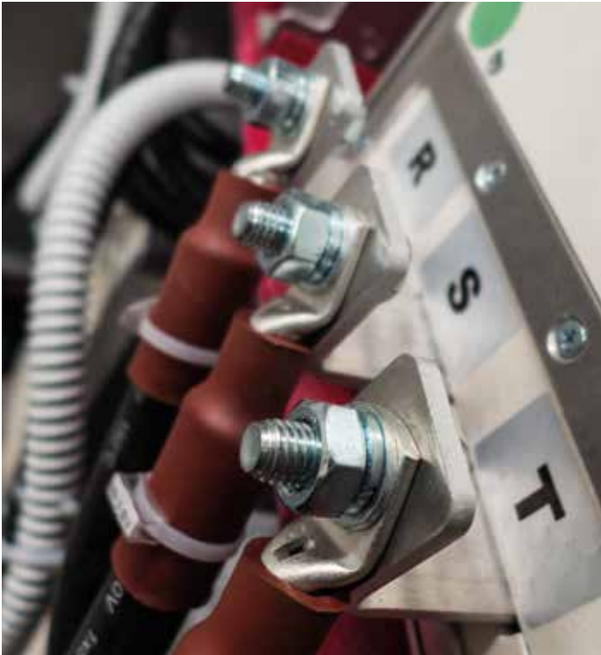
CHB-cell converter detail - 6 pulses input diode bridge
